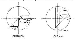
Diagram showing chamfer and radii dimensions on crankshaft 99-306549 which must be adhered to when crank grinding is undertaken.
